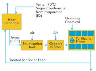
Treated Condensate for Cooling Tower Make-up
